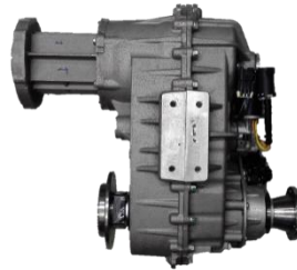
Dual – offset Transfer Case with bevel differential
