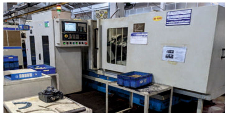
Retrofitted HMTLiebherr H400 Gear Hobber
