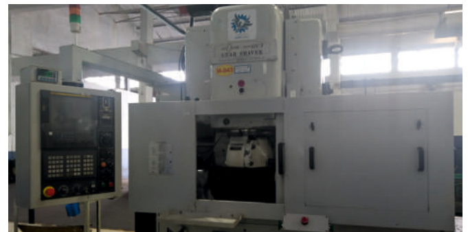
Retrofitted Red Ring Gear Shaver - ARK
