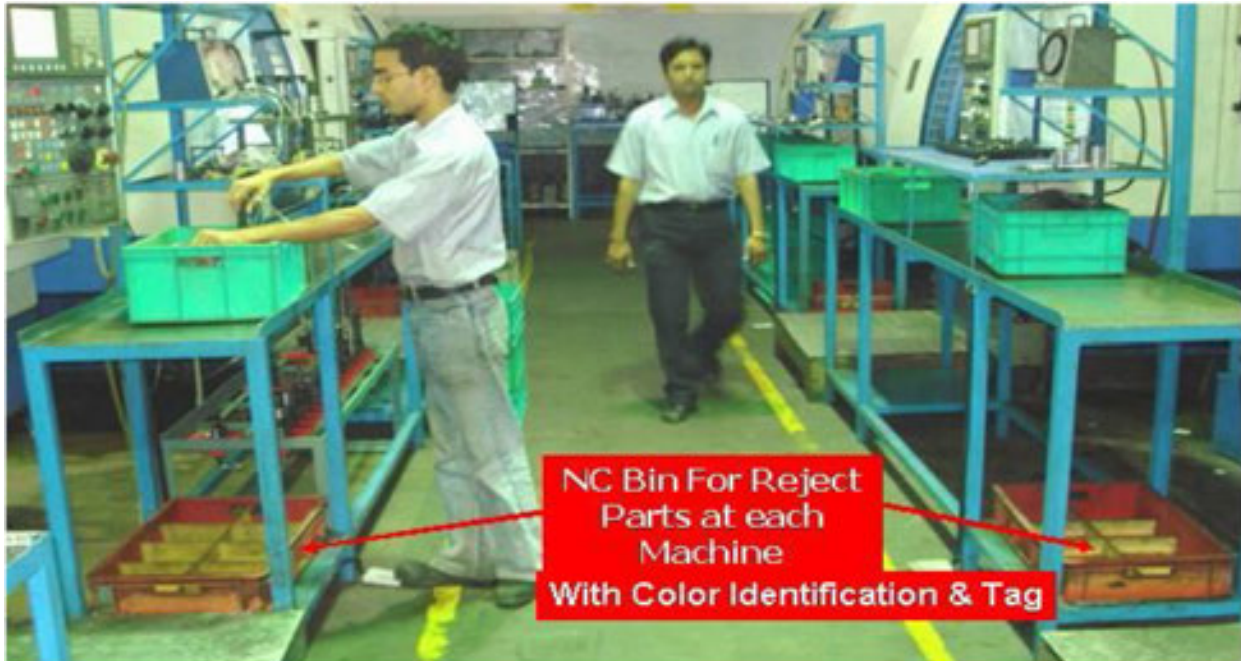
Figure 10. Control of Non Conforming Product
