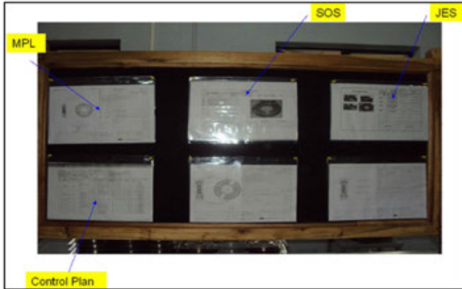
Figure 14. Standardized Operation Display Board
